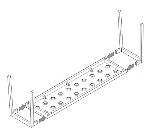
Secure the legs with screws **B** and Allen key **C**. Tighten all screws lightly before tightening them all completely.
