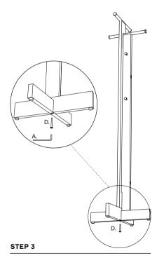
Mount the last screw (D.) to the bottom of the Foyer Coat Stand.
